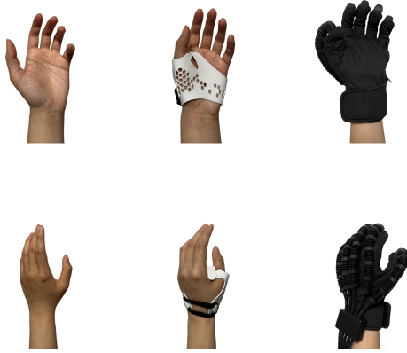
Fig. 4. Hand configuration comparisons: (a) bare hand, (b) hand with 3D printed thumb brace, (c) complete orthosis glove worn over thumb brace. The brace maintains functional thumb positioning while allowing pneumatic flexion.
